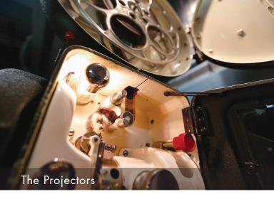
A gift of the Century Projector Company, the Century Model C projectors have been installed in the Dryden Theatre since it opened in 1951. These machines are "closed head" projectors, so called because the entire film path from feed magazine to takeup magazine is enclosed. This makes them safer for running nitrate print film.
