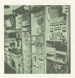
ANALYZER. This complex instrument uses digital television techniques to extract and record the first-, second-, and third-order probability distributions of pictures on magnetic tape. This kind of statistical information is used in designing more efficient visual communication systems.
