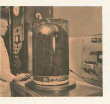
VACUUM EQUIPMENT FOR DEPOSITION OF THIN FILMS. This laboratory contains complete high-vacuum evaporation systems for the controlled deposition of thin coatings of both metallic and dielectric films.
